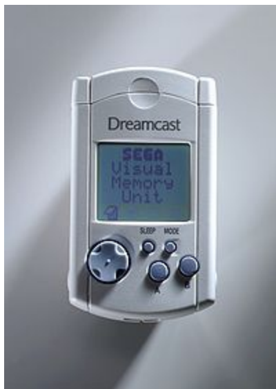
Close-up look at the VMU while run in standalone mode. It's powered by 2 CR2032 batteries.
